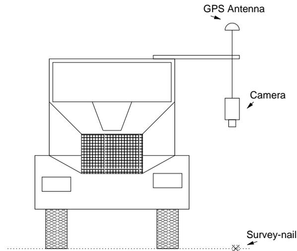
Figure 3: Measurement Setup for Evaluating the DGPS
